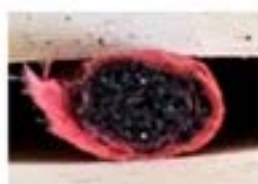
Cross section of a commercially available sparkler
